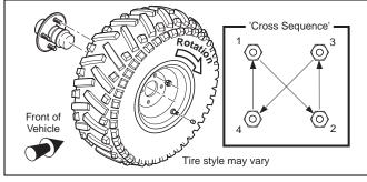
Fig. 17 Wheel Installation
